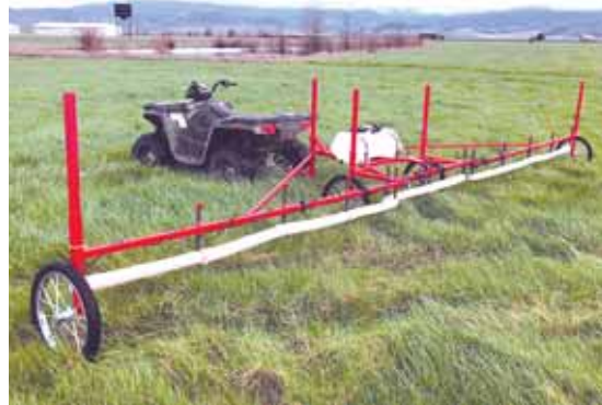
Wheels at each end keep the boom at specific heights, which are fully adjustable based on in-field weeds. The sponges evenly distribute chemicals across the boom to thoroughly coat every weed it comes in contact with.
