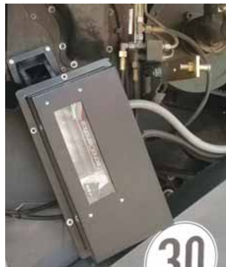
Mounted on a combine, Grain-Q makes it possible for the operator to identify and harvest areas with uniform grain qualities, such as certain oil levels in soybeans, protein in wheat, or starch in corn.
