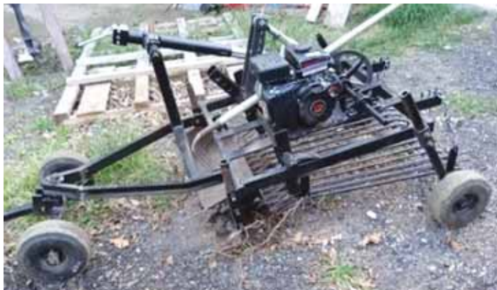
Brahn built his digger with a 3-hp. motor to run the digging pan and shaker.
