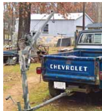
Engine hoist fits a 2-in. Reese hitch receiver.
