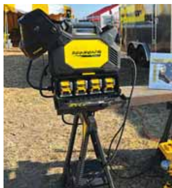
Four 12 Ah batteries can burn up to 33 (E6013) electrodes on a single charge.
