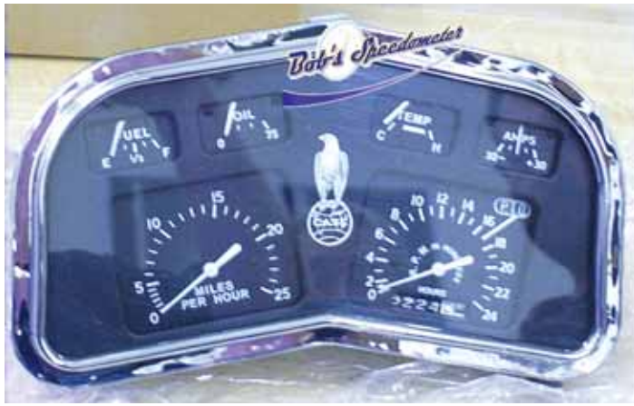
Restored instrument cluster from 1962 Case tractor.
