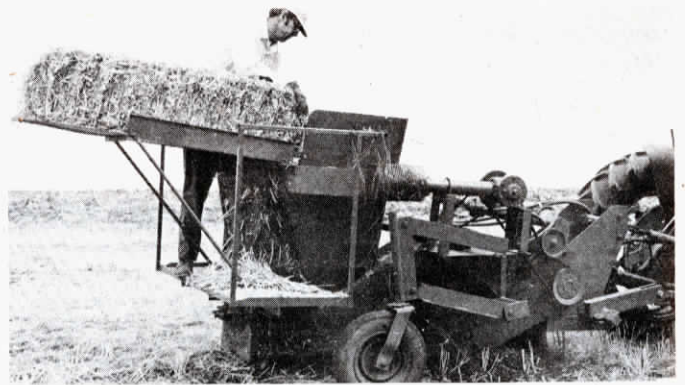
Researchers developed mulching machine to fill trenches with straw to increase water infiltration and reduce erosion.
