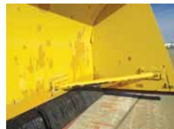
Schuyler makes its laminated cutting edges by compressing rubber sections onto 1 1/4-in. steel rods and securing them every 12 in. with fault bar retaining plates.
