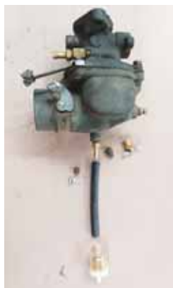
300 IH carburetor with drain line, filter, and brass drain valve.
