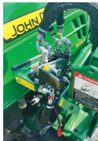
Single-point hydraulic connectors like those used on large Deere equipment are now available as an optional kit for the Deere 120R loader that mounts on smaller diesel tractors.
