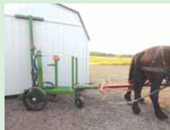
Shed mover has a 12,000-lb. lifting capacity and comes with either a tractor hitch or a tongue for horse towing.
