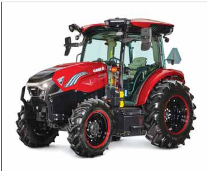
Farmall 75C claims a 4-hr. run time before charging is needed. Three recharging options are available.
