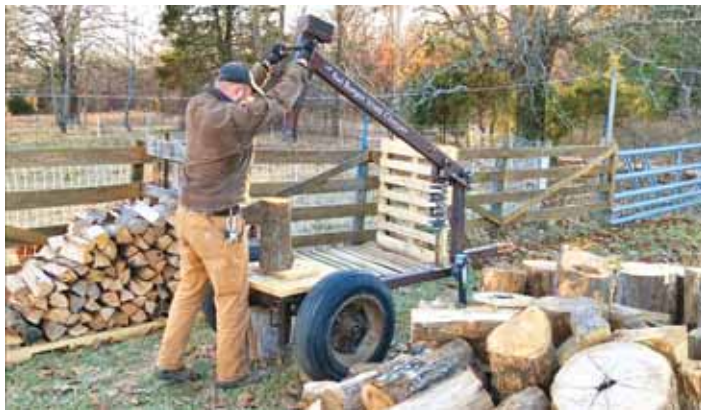
Wylie made the splitter largely out of salvaged metal, using an old boat trailer tongue for the frame and setting it on a mobile home axle.
