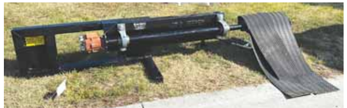
EZ Sweep features a durable frame with a high torque, low-speed hydraulic motor that rotates treaded rubber mats forward to whisk out any debris within the bunks.
