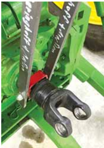
Decoupler flange tabs in place against coupler end.
