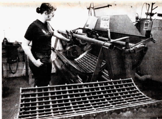
Hardfacing quadruples effective life of a concave, according to Farrar Corp., which also hardfacing combine cylinder bars.
