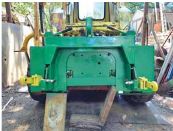
Bracket has holes for two bolts. The pin that locks into the pin hooks on the quick attach plate goes through one hole. A nut secures its threaded end to the bracket.
