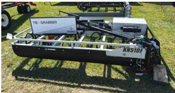
“Tie-Grabber picks up a group of bales and ties it off before setting it on a transport,” says Kuhns. “It makes the tied groups more stable for vertical stacks that won’t fall over.”
