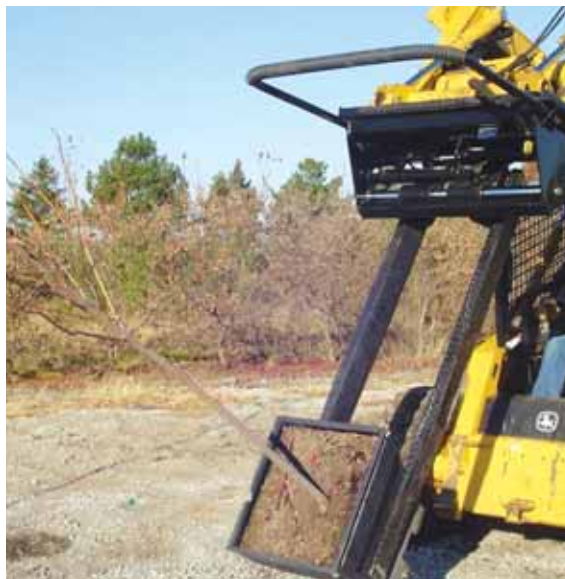
A heavy-duty double cylinder moves both forks in or out as desired. The forks lay flat to be used as regular pallet forks but are hinged in the back to rotate to the perfect grabbing angle.
