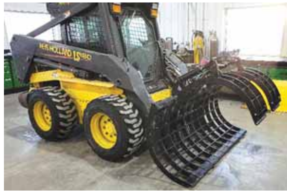
Madsen's grapple works well for jobs like clearing trees, and back blading gravel as the rocks flow through the holes in the concaves while driving.
