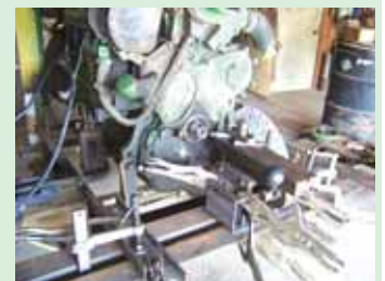
Jig held in place with clamps and vice grips.
