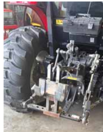
Streenz built a handy 3-pt. attachment with two large hooks to carry garbage bins.
