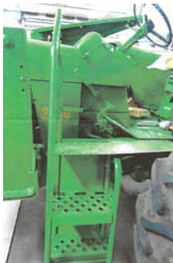
First step is 16 in. off the ground, and the handrail on the side makes them act more like stairs than a ladder.
