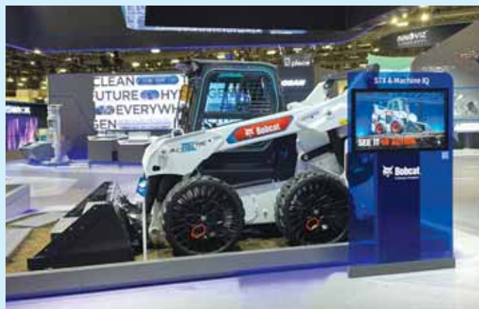
"The first thing customers notice is the instantaneous torque, up to three times greater than traditional skid-steer loaders," says Honeyman. "Our peak mode lets an operator go from 75 hp. to 107 hp. when driving into a pile."
