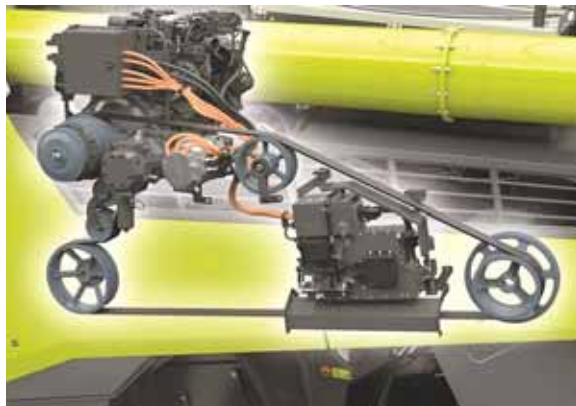
Lexion e-hybrid system connecting to diesel-powered drivetrain.
