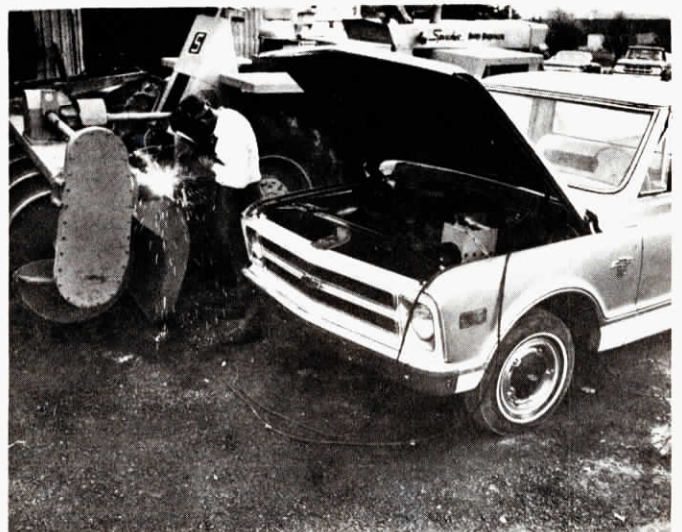
Welder uses high frequency instead of amperage to heat metal.
