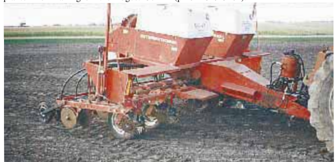
Link mounted new Yetter row cleaning wheels on front of planter. Each pair of wheels clears a strip wide enough for two row units.
