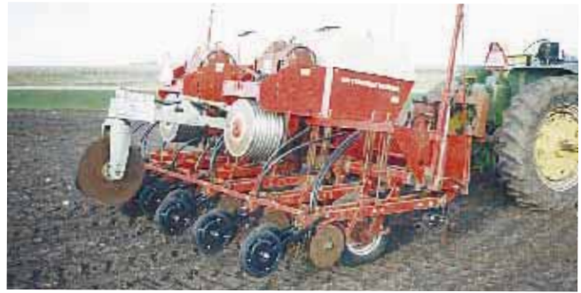
The 6-row planter plants two rows 7 in. apart on top of ridges and is equipped with a single blade Orthman automatic guidance system on back.
