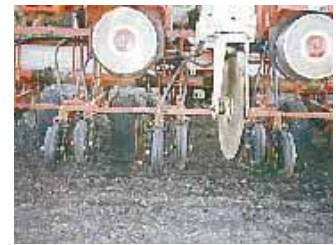
Add-on row units mount on separate brackets behind and 7 in. to side of original row units.
