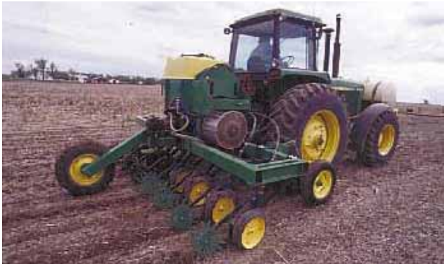
Gillen built a frame for a Cyclo air seeder and fitted it with disc openers off a Deere 750 no-till drill. When finished he painted the 8-row planter Deere green.
