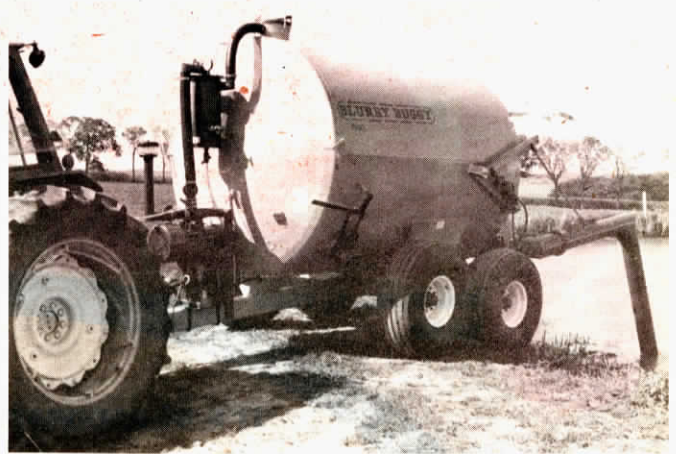
The 2,900 gal. tank fills itself in just 4 min. or less.
