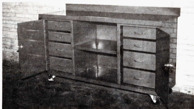
Top of portable toolbox-workbench is heavy enough to support a vice.
