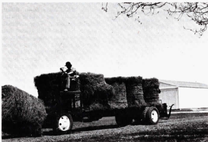
Miles' bale bus picks up bales on the go at 5 mph and transports them down the road at 50 mph.
