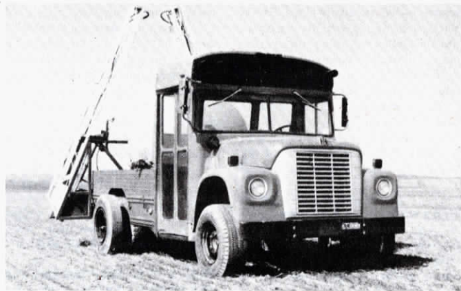
Pluhar's school bus sprayer has a 750 gal. tank and a 60-ft. boom.
