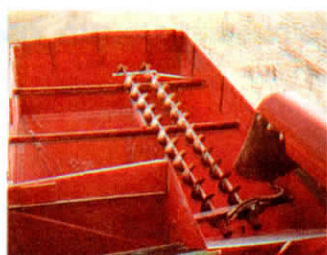
A pair of small leveling augers driven by orbit motors mount across top of cart.
