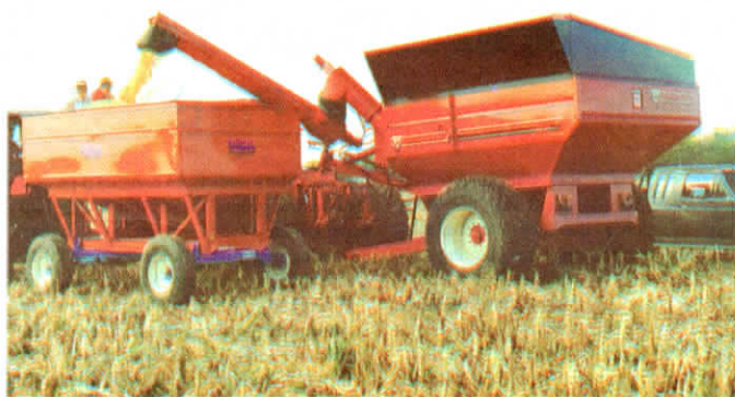
Cart has two separate sections of auger, each driven by its own hydraulic motor.
