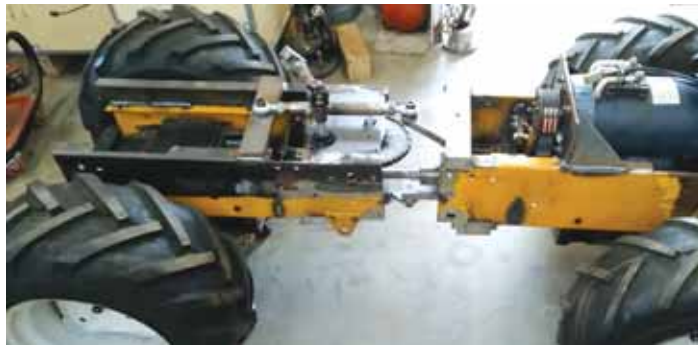
Articulation, steering and direct drive assembly were some of Bayer's challenges.
