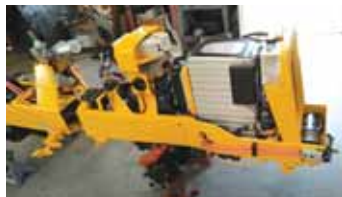
Final assembly with battery pack, electrical and steering in place.
