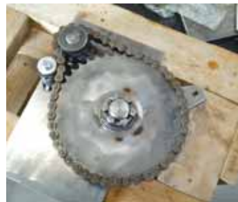
Steering chain drive with sprockets (above) and lithium-ion battery pack (below).
