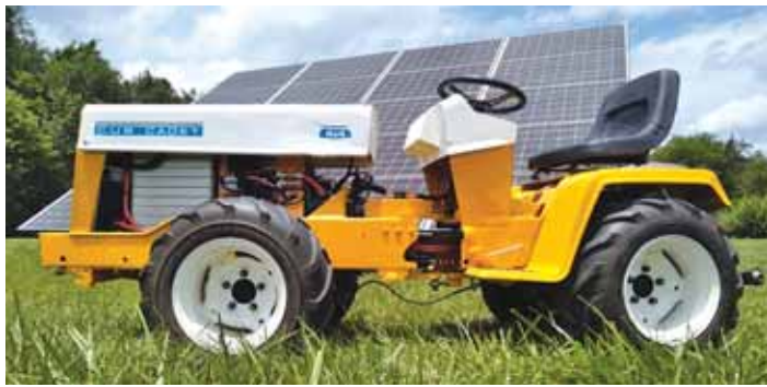
Bayer created his eCub using two scrap Cubs, a golf cart motor and a Nissan Leaf car battery pack.
