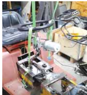
Steering wheel and assist motor were suspended above the shaft from the chain drive.
