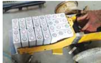
Steering chain drive with sprockets (above) and lithium-ion battery pack (below).
