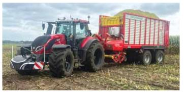
Air bumper weighs 600 kg. (1,320 lbs.) and doubles as a front-end weight block. The system can also be used with an air gun to control excessive dust build-ups on other equipment.
