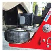
"These air-ride hitches control the chucking back and forth to settle everything down. It's the best of both worlds when traveling over rough roads, railroad tracks, bridges or other rough terrain," says Watson.
