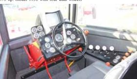
Cab interior was completely refurbished during restoration. Above the console, a monitor in front of the driver showed the implement being pulled.
