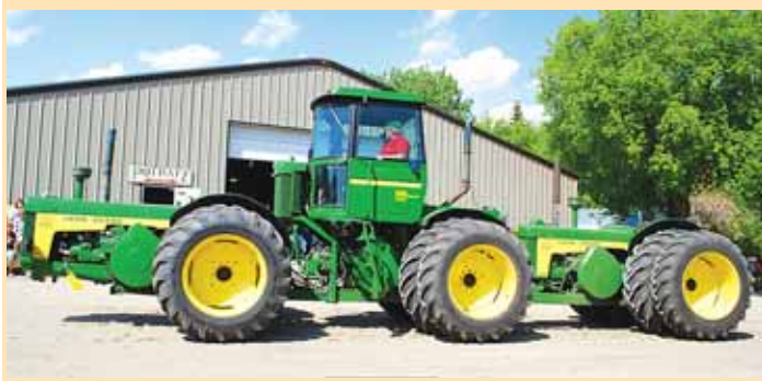
Dufner's "830 Special" is a 6-WD powerhouse that uses three 830 engines to produce 300 hp.
