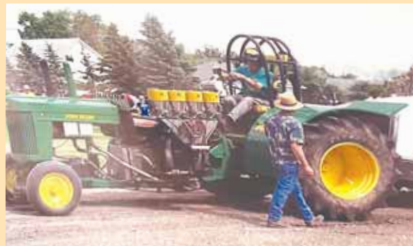
Dufner put an Allison aircraft engine on a Deere R frame, creating a tractor-pulling monster.
