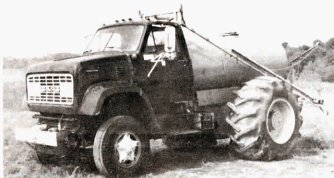
Greg Ellerman's "Truck-Tor" consists of a GMC chassis, cab, and front-end combined with a 50,000-lb. payloader rear axle.
