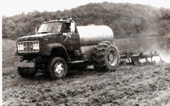
The truck-tractor combination is at least equal to a 150 hp. tractor, according to Ellerman.
