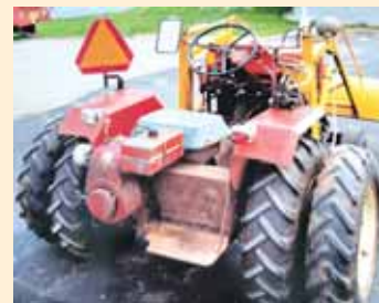
A small red engine on the back of Earl Zuleger's shop-built tractor was his way of creating live hydraulics to raise and lower attachments.
