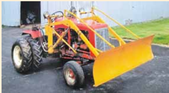
Mounted plow was from a David Bradley walk-behind tractor. His son Duane added the dual wheels.
