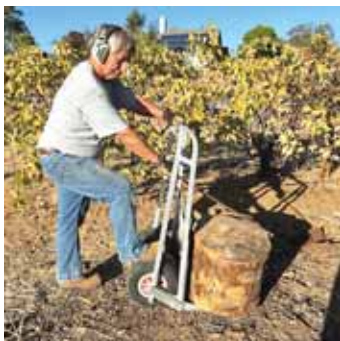
Toso made his own cart to move heavy logs, including a rebar hand hook for loading.
