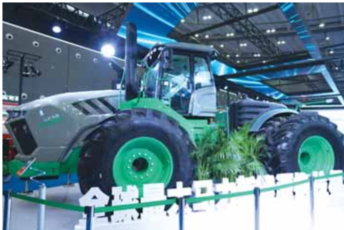
Tractor's innovative E-CVT system combines a mechanical transmission with an electric one, allowing the engine to operate more efficiently.
