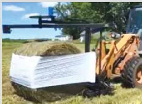
**Bale Buddy 2000** by Halverson Wood Products ([www.halversonwoodproducts.com](http://www.halversonwoodproducts.com)) was designed to allow hay to be baled with up to 60% moisture, saving time waiting for drying and saving on spoilage.
