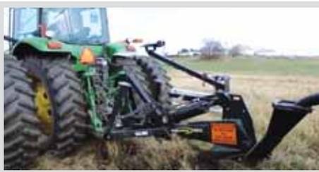
**Soil-Max Stealth ZD** ([www.soilmax.com](http://www.soilmax.com)) Requires an 8,000-lb tractor and can install 2 in to 4-in. tile at up to 4 ft. deep. Manufactured from T1 steel for greater strength with less weight. It has a proprietary proportional valve for adjustments and has poly sides for easier pull. They have an online ROI tool to see if it's a good fit for your farm.
