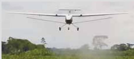
**Pelican Spray** ([www.flypyka.com](http://www.flypyka.com)) An autonomous electric aircraft designed for ag, it has chemical drift reduction technology and can carry a 620-lb. payload. Lidar/radar capability make it useful at night. With a 38 ft. wingspan and 60 ft. wide spraying capability it brings a new option to aerial spraying.
