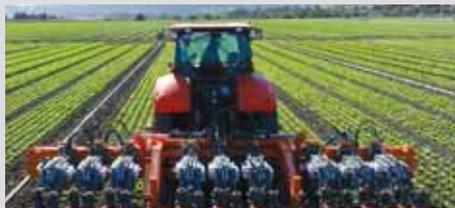
**FarmWise Labs** ([www.farmwise.io](http://www.farmwise.io)) The Vulcan T380 AI-driven weeder was developed for the tomato processing industry. Using computer vision it can locate stems and eliminate weeds around plants at speeds of 2 to 4 mph.
