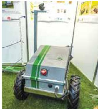
**SmartFence** robot uses a 3D camera to identify the stakes and wire. Then, it analyzes the fence and cuts any growth below.
