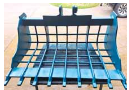
Gunn's shop-built rock rake.
