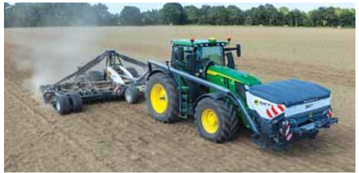
Two large compartments hold up to 1,100 liters of seed and fertilizer, while the smaller front and rear sections hold 100 liters of product.
