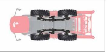
Combination of the suspension system and the chassis design eliminates cross-distributed movements in the main frame and, more importantly, in the boom, which causes boom yaw.
