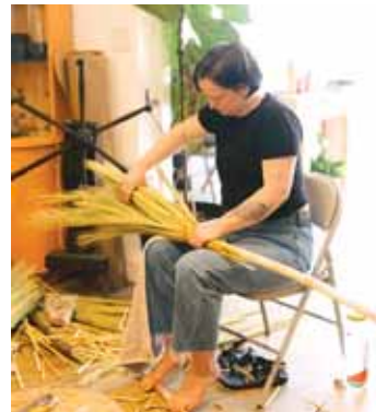
"Homemade brooms can include the 'split ends' or fines of the top of the crop (called the hurl)," Main says. "It makes them better at grabbing dirt than factory brooms."
