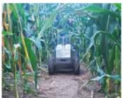
Upside Robotics developed the Maize Runner, the first live-in-field robot. The 24-in. wide electrically-driven miniature robots are sized to fit between 30-in. corn rows, spraying liquid fertilizer directly onto the plants right in season.
