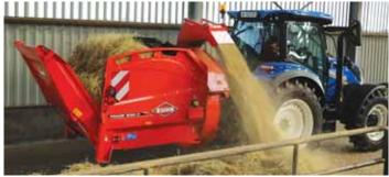
Primor 2060M options include a secondary remote controller to raise and lower the tailgate from outside the cab and a 300-degree swivel blower chute that sends bedding 60 ft. to the right and 42 ft. to the left.
