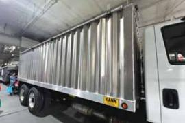
Kann trailers are unique because they're built with all-welded construction from 1/8-in. continuous corrugated aluminum walls.
