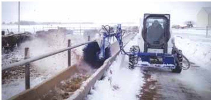
Feed Bunk Sweeper is designed for skid steers and small wheel loaders. Its manually adjustable arm with telescoping boom has a poly bristle broom.
