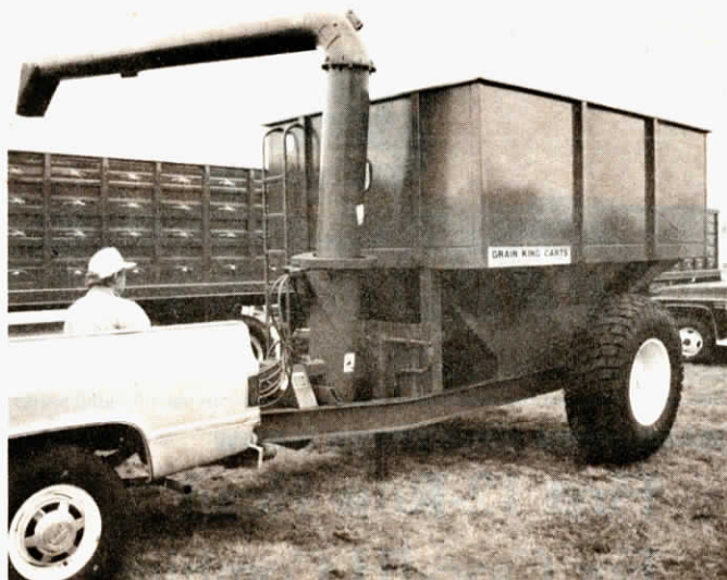
The auger turns 360° and will unload 400 bu. of dry grain in 3 1/2 min.
