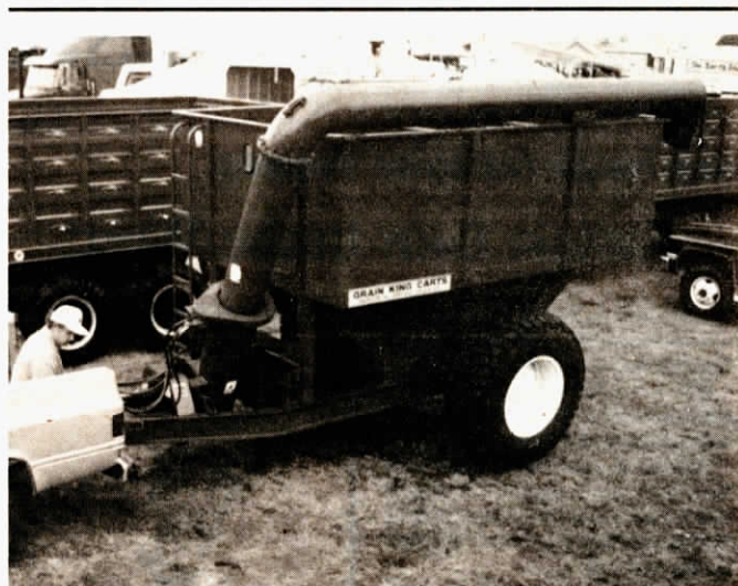
The auger can be used to aerate grain by closing up the spout and extending it back over the wagon. Wet grain circulates up through the auger and drops back into the wagon through a series of holes that open up on the bottom side of the auger.
