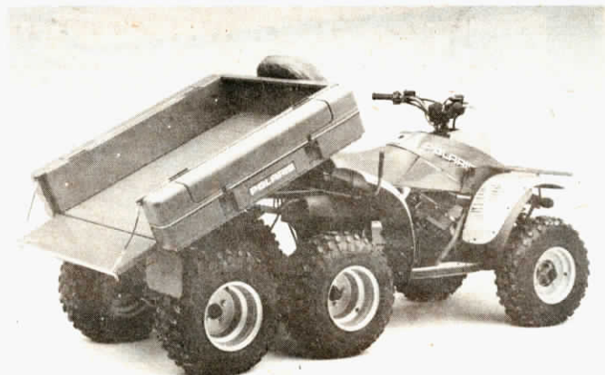
There are toolboxes on each side of the 600-lb. capacity cargo box.
