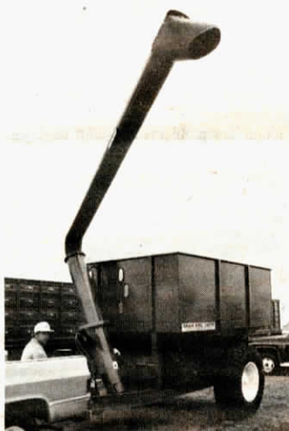
The auger also pivots 2 ft. from side to side, allowing it to be lowered to within 18 in. of the ground or raised 18 ft. high.
