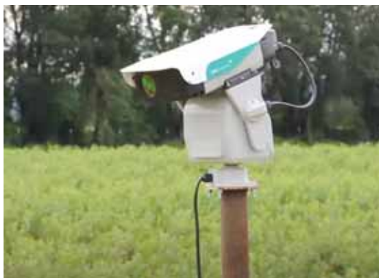
One AVIX Autonomous Mark II can deter birds from 15 to 20 acres.
