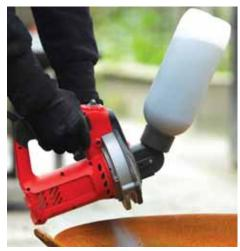
A high-speed wheel creates the pressure. Blasting medium gravity feeds into the airflow from the abrasives container. Equipped with a laser pointer, the handgrip, with its protective shield, directs the flow to the target.
