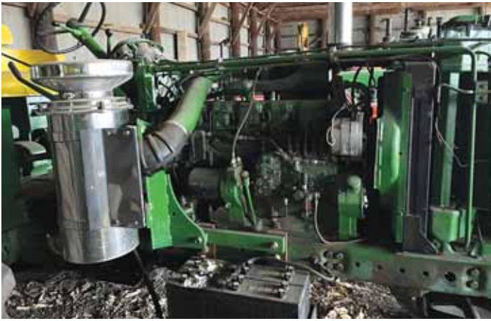
Bauer repowered a 4020 Deere LP model with the turbo diesel engine from a 7700 Deere combine.
