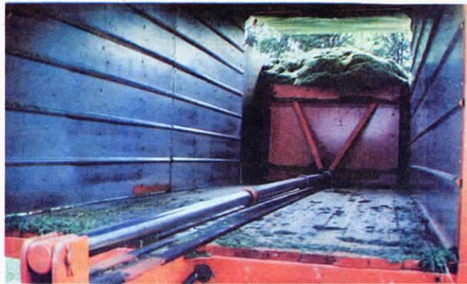
Hydraulic ram can be activated as load is being chopped to compress it and thus increase carrying capacity. When box is full, ram pushes load out.
