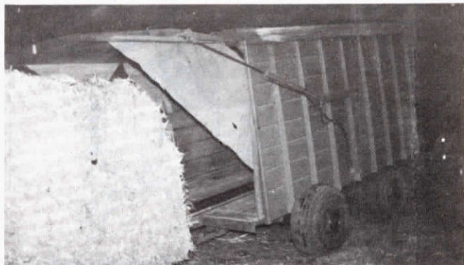
Rear axle of chopper wagon lowers hydraulically for "pushing off" loads directly onto the ground.
