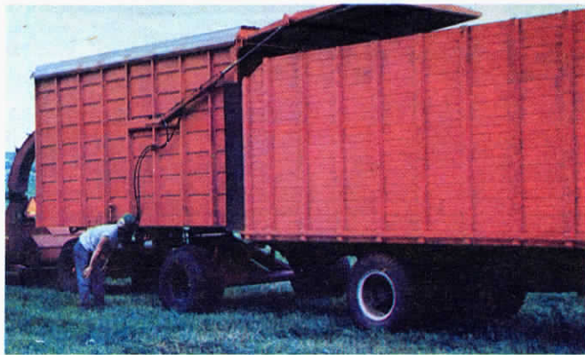
Bed of chopper wagon, left, can be raised or lowered hydraulically via "floating" rear axle to line up with truck bed for "push off" transfer of the load.
