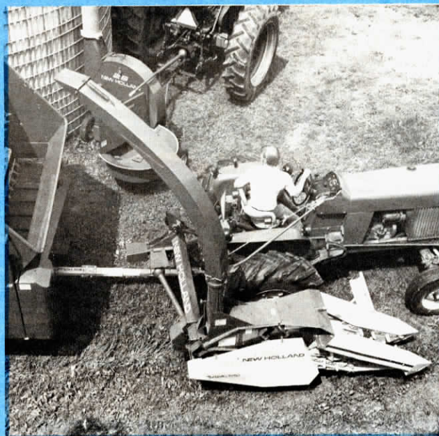
New Holland's 707 has up to 26 tons/hr. capacity.
