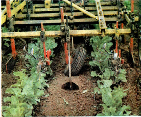
Inventor Paul Bezzerides, right, with basic unit consisting of "tilted" gauge wheel and guide furrower. If guide wheel on right side of cultivator is mounted to tilt to left, opposite side guide wheel must be mounted to tilt right (or vice versa). Photo on left shows leveling shoe traveling behind tilted guide wheel.
