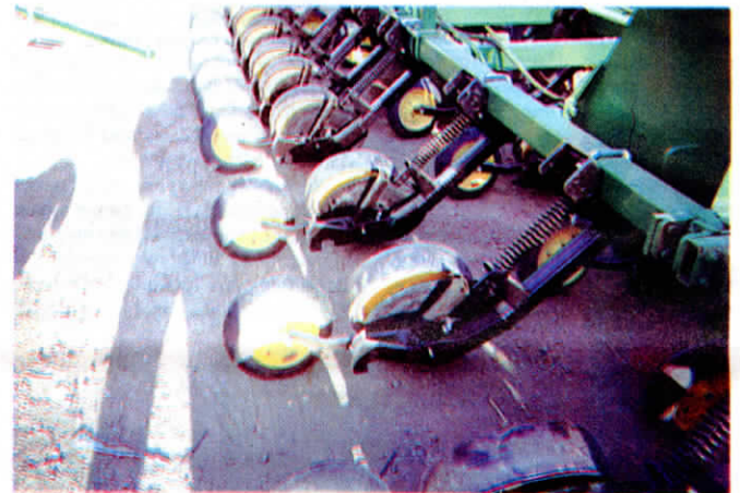
Add-on row units replace existing field cultivator shanks. A single disc opener is set at a 23° slant and turned at an 8° angle to direction of travel to make opening.
