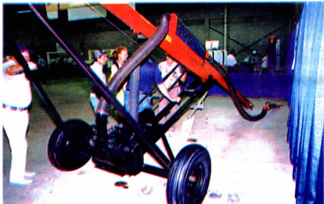
Auger is fitted with both conventional flighting and with a grain vac, making it ideal for cleaning out bins or moving grain out of flat storage.
