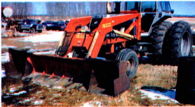
Yarema added 2 1/2-ft. extensions to either end of Leon 8-ft. wide bucket.
