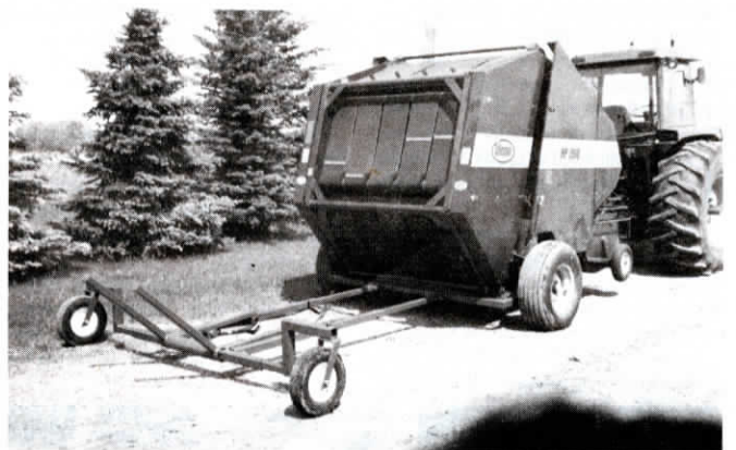
Fitted with caster wheels, cradle bolts to frame so it becomes integral part of baler.
