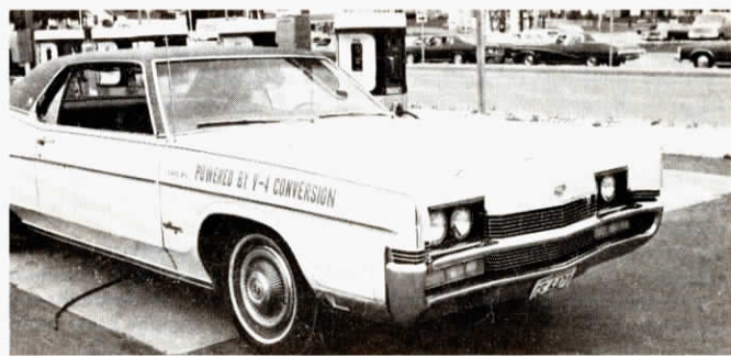
This 8 cyl. car, which Lucia converted to run on only 4 cyl., gets about 100 more miles per tankful of gas.
