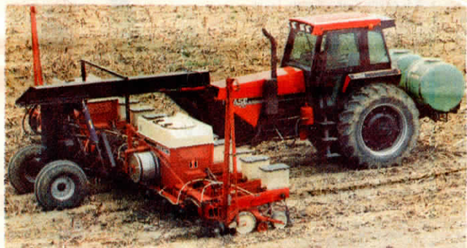
With 12 row equipment mounted up front instead of behind, the front tractor wheels (moved 10 ft. forward) directly control the equipment.
