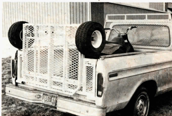
Ramp/trailer folds up into a vertical position for transport. When not needed, ramp can be removed leaving a gas-saving "shorty" tailgate in place.
