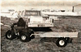
Slip-in tow hitch quickly converts ramp to a 1,000-lb. capacity trailer.
