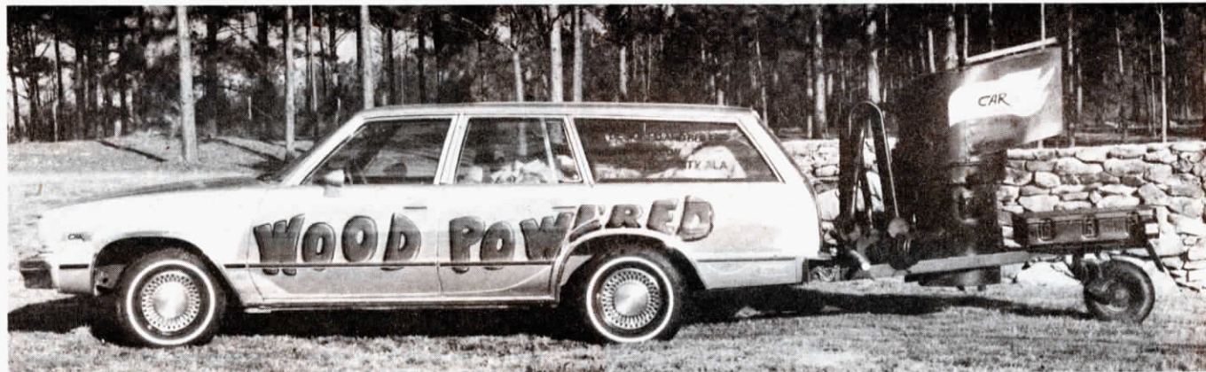
This specially-rigged Chevy station wagon traveled from Florida to California on wood fuel. The wood-to-gas generator trails behind and powers the car about 150 mi. per 100 lbs. of wood.
