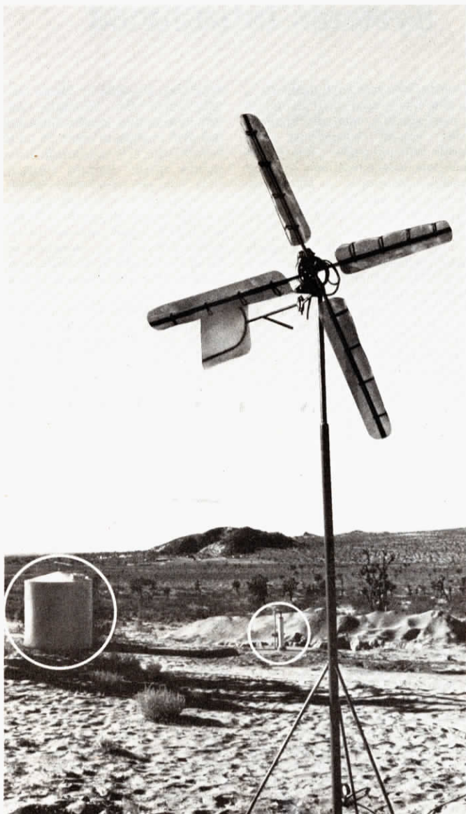
Capacity of the new Bowjon wind powered pump is right at 5 gpm. Air compressor built into head pumps air through flexible tubing leading to well. Air injection lifts water to tank or pond. Windmill doesn't have to stand over well or water source.
